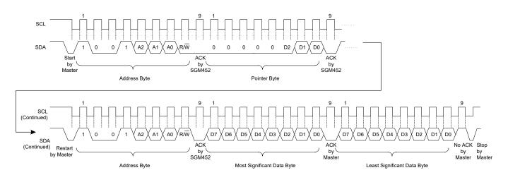
(b) Pointer Set Followed by Immediate Read for 2-Byte Register Such as Temperature,  $T_{OS}$  and  $T_{HYST}$
