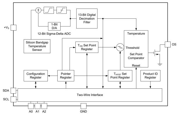
Figure 5. Block Diagram
