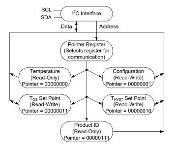
Figure 8. Register Structure
