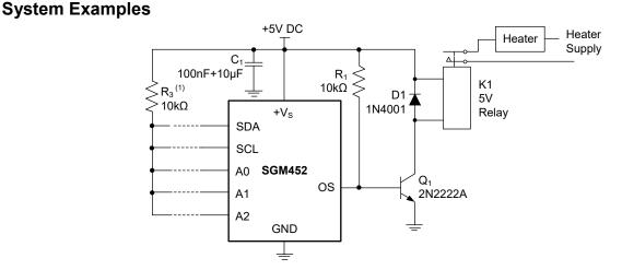
Figure 10. Simple Thermostat, Interface Optional
