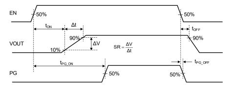
Figure 3. Timing Diagram
