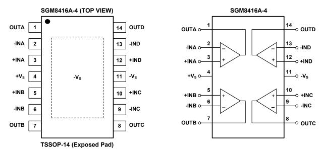
NOTE: Connect thermal die pad to -V<sub>S</sub>. Connect it to -V<sub>S</sub> plane to maximize thermal performance.
