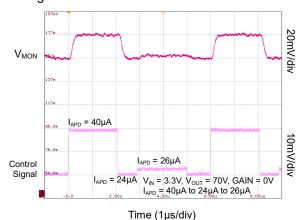
Figure 5. Burst Pulse Receiving Waveform
