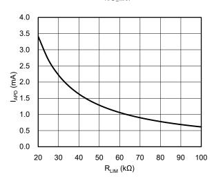
Figure 3. APD Current Limit vs. RLIM
