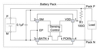
Figure 1. Typical Battery Pack Circuit
