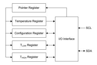
Figure 12. Internal Register Structure
