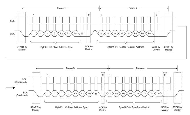
Figure 5. Register Read Byte Format
