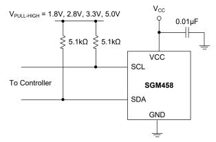
**Figure 8. Typical Connections**
