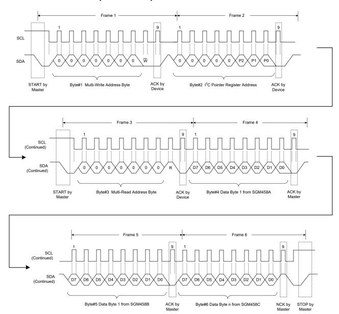
Figure 7. Register Multi-Read Format Using in Typical Application
