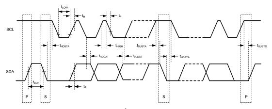
Figure 3. I<sup>2</sup>C Timing Diagram
