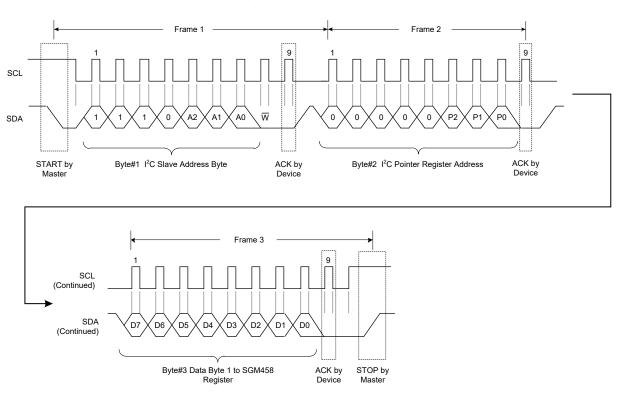
Figure 4. Register Write Byte Format
