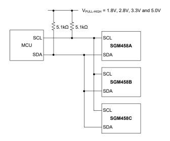
**Figure 1. Typical Application Circuit**
