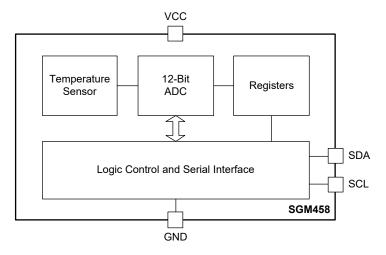
Figure 2. Block Diagram
