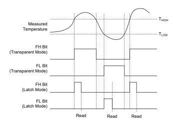
Figure 9. Temperature Flag Functional Diagram
