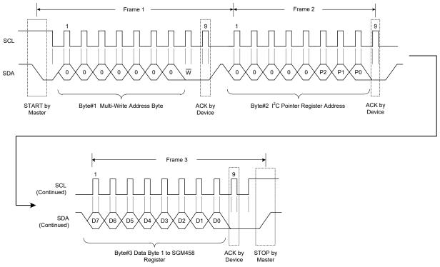
Figure 6. Register Multi-Write Format
