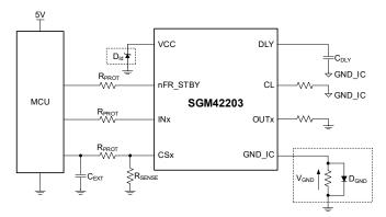
Figure 1. Application Schematic
