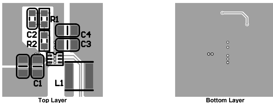
Figure 4. SOT-563-6 PCB Layout
