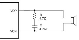
Figure 5. RC Snubber Circuit
