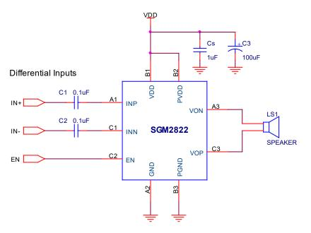
Figure 6. Differential Audio Input (for Mobile Phone Application)
