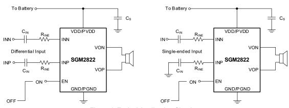
Figure 1. Typical Application Circuits
