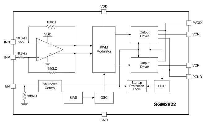
Figure 3. Simplified Function Block Diagram of SGM2822
